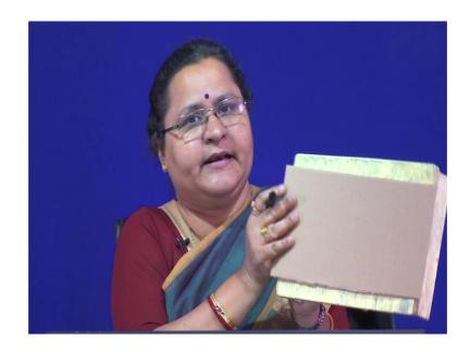
So, if we have a system like this; you can put it put your absorbing material directly on it you can put it put directly on it or you can put it with an air gap. So, if you can put it with an air gap; you will get the advantage of having the air in between.
