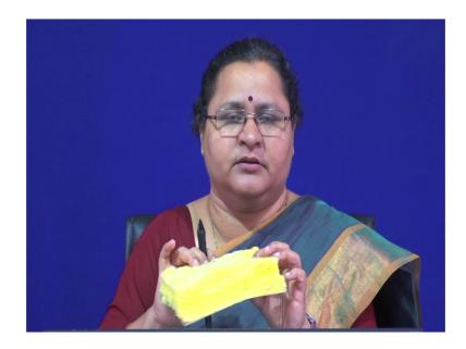
So, this is what is mineral fiber, which can be used as an absorber but as you all know to other subjects that this is made of glass this is sorry; this is glass fiber and these are very fine fibers of glass which cannot be kept exposed.
