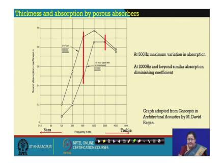
And we are getting almost close results with the different thicknesses when we are at around 1000 hertz of frequency. So, it matters the thickness matters when we are trying to tap; while we are trying to absorb sound between 250 to 1000 hertz and around 2000 hertz this thickness really does not matter.
