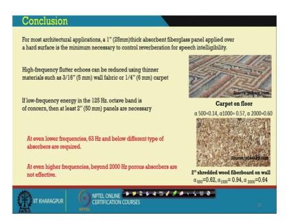
So, what we can conclude is for most architectural appliances applications 1 inch that is 25 millimeter thick absorbent fiber glass panel applied over a hard surface is the minimum necessary to control reverberation; for speech intelligibility.
