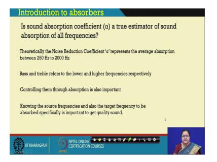
Now, we have told you regarding Professor Bhattacharya has told you regarding sound absorption coefficient, which is an estimation of how much sound how much sound can be absorbed by an object. But is it a true representor or true estimator of the sound absorption of all frequencies may not be at all cases.
