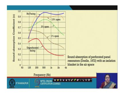
And as I told you the amount of perforation do have a bearing, but up to beyond 15 to 20 20 percent of perforations is acceptable and does not hampered the sound entry is well demonstrated through this graph. So, you see one is having unperforated facing that is something which is solid, which is facing it at the same time we see that with no facing which is the top blue line is almost matching with 13 percent opening which is the orange graph just below it.
