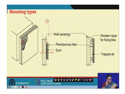
So, how can we; so coming to the mounting type if you are mounting it with an air gap; you can actually take the advantage. Whereas, if you mounted directly to a structural system by testing it with an adhesive, you get a different curve; so that is what has been demonstrated what is that is what has been demonstrated here.
