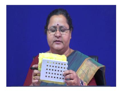
So, we can actually cover it with a porous of with perforated surface which can come on top of it and it can actually hide that material behind you.
