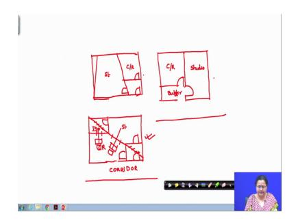
So, if we have a simple rectangle and here is a corridor and here you have to plan your recording and the studio and the recording control room and recording room. You can go for such buffer space and this is your say the control room or and this is the studio. But the problem here is the proportion is may not be achieved, it is suggested that in the same space we could have planned something like this.
