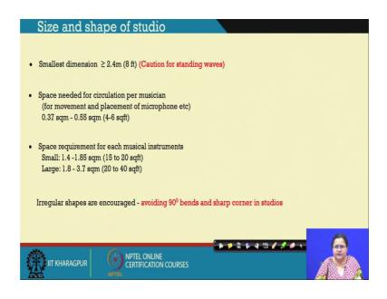
Now as architects we believe that first we have to plan for the space. So, we need to know the size and shape of the studio. So, the smallest dimension suggested is 8 feet or 2.4 meters and greater than that is acceptable and here the caution is for standing waves. Because you can understand these smallest dimensions and dimensions nearer to it are actually under the small rooms and here standing waves can be happening. Space needed for circulation per musician is kept as 4 to 6 square feet.
