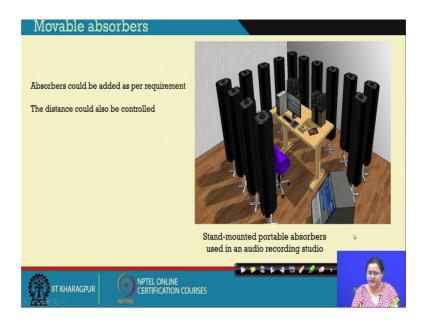
Here you have the movable absorbers, it is the same slide where absorbers could be brought in or taken out as per requirement. Their distances also could also be controlled and these are stand mounted portable kind and this could be also acquired to get a to achieve a particular reverberation time.
