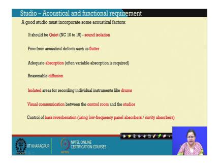
So, basic requirement towards function and towards acoustics are to have a quiet isolated area. So, I have already mentioned in one time during classroom the NC curve 10 to 15 is to be followed NC curve will be dealt with Professor Bhattacharya. Free from acoustical defects that is having parallel walls causing of flutters, and such kind of defects are to be avoided, adequate absorption by using different absorbing materials can be adapted.
