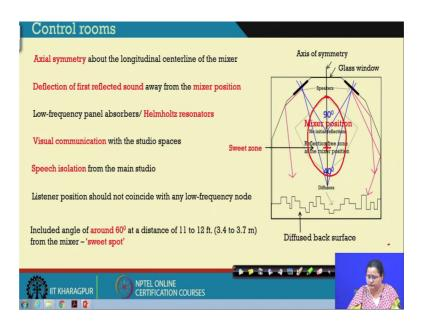
Coming to the control room this area is totally controlled by electronic devices which we are not expert in we are only to keep the plan for the space. So, what we see here is the axis of symmetry is to be kept to locate the speakers, and this axis of symmetry is for the mixing area.
