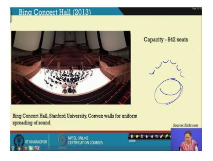
This is a very recent hall with a very small capacity 842 made in 2013, where you can see on the sides there are a number of number of convex towards the stage, wall surfaces and the ceiling over is also a convex surface. So, the ceiling is looks like a kind is very circular and on top of it where these all goes and merges the ceiling is hold over there.
