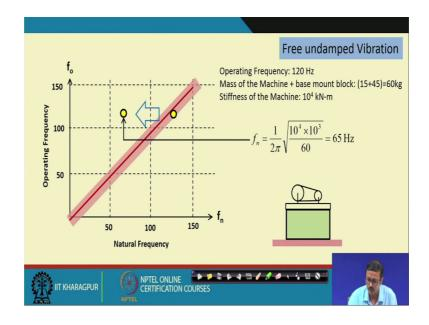
So, what I did is that I change the mass which was actually 15 here, the mass of the machine and which is rested on the slab itself. Now I put a the heavy mount system and the mass is now suppose 60 kg and if it is 60 kg and the stiffness remains unchanged this f m that is the natural frequency become 65 Hertz and now the this 130 Hertz from here, it is move to the 65 Hertz and the operating frequency remain unchanged 120 and this is your 65.
