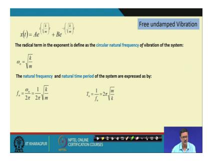
We can find out there is r radical which is under root k by m is nothing but the circular the natural frequency of this particular vibration vibrating system. And definitely it will be a circular natural frequency is there because this particular vibration motion of the vibration is the sinusoidal kind of thing or is a kind of a the simple harmonic kind of thing.
