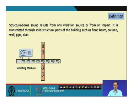
The structure-borne sound by definition is as we already discussed in lecture 31 is a there are two way a sound propagate from one place to another; one through the air which is the borne sound transmission and for that we need to develop some kind of a transmission loss. Suppose from source room to the receiver room, some sound is propagating.
