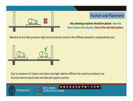
The next one is that the vibrating machine should not be placed in the center of the slab, I mean if at all you want to place it in a in a in a upper floors because many times we cannot aware that particular vibrating machine to be suppose a choose or each and every floor you have to give some kind a choose and which is have been some kind of a pump or some kind of a the diffuser.
