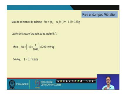
So, I have to increase the mass it mass, actually 3.9, but this has to be 4.8. So, point 9 k g or 900 gram of the mass has to be increases this particular plate. So, how can increase the 0.9 k g of the mass by virtue of some application if some kind of a thick metal paint paints?
