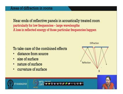
Now let us come to the areas of diffraction in a room. Near ends of reflective panels in acoustically treated rooms particularly the role low frequencies which have large wavelengths the wavelengths actually bend. There is a loss of reflected energy of those particular frequencies and you can actually not get those particular frequencies towards the listener.
