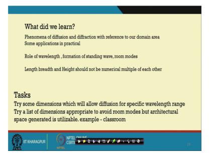
The phenomena of diffusion, diffraction with reference to our domain area, we have also talked of some application in practical, we understood that the role of wavelength is so very important in the formation of standing waves and room modes, it is also very important in the phenomena of diffusion and as well as diffraction. But that was not much of important when we were dealing with reflection.
