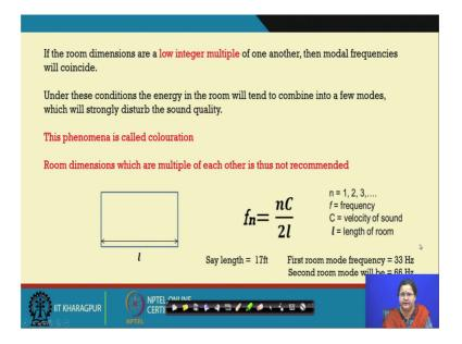
So, this phenomenon is called coloration. And room dimensions which are multiple of each others are not at all recommended.
