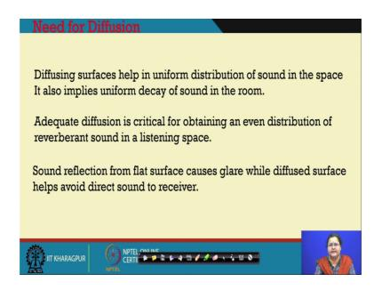
So, what is the need for diffusion? Diffusion helps in uniform distribution of sound in the space and it also implies uniform decay of the sound with in the room. So, it actually distributes the sound energy equally towards the receivers all from the front in the back. Adequate diffusion is critical for obtaining and even distribution of reverberant sound in
