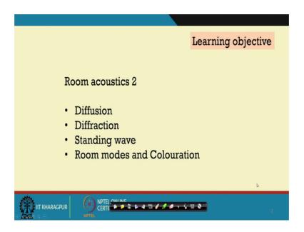
So, we will come to the Room Acoustics part 2 which will deal with the diffusion of sound, diffraction of sound, standing waves, room modes and coloration. So, I have given a basic understanding of what is diffusion- that is scattering of sound, diffraction-that is bending of sound but not on the other two.
