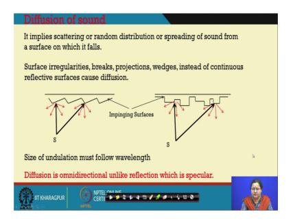
So, diffusion implies the scattering of sound or random distribution of spreading of sound from a surface on to which it is falling. So, it is taking place in all direction it is not only the specular reflection which was happening in case of reflection in one direction.
