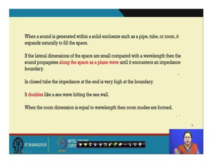
So, if we see that when sound is generated within a solid enclosure; say such as a pipe or a tube or in our case a room it expands naturally and fills up the space. So, the space in front of me is filled up by the sound energy which is thrown by me or by my voice.
