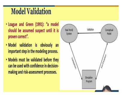
Okay. Now the next important aspect is model validation. Now, you know that a model should be assumed suspect until it is proven correct. So this diagram shows the model validation practice. So model validation an obviously an important step for modeling process, model must be validated before they can be used with confidence in decision making and risk assessment process okay.
