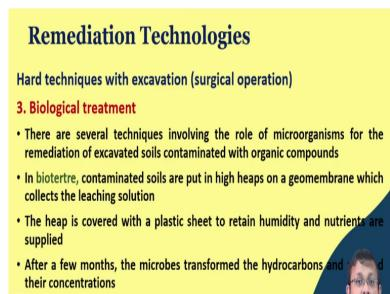
Now, there are several techniques involving the role of microorganism for the remediation of excavated soil contaminated with organic compounds. In biotertre, the contaminated soils are put in high heaps on the geomembrane which collects the leaching solution and the heap is covered with the plastic sheet to retain the humidity and nutrients which are basically supplied.
