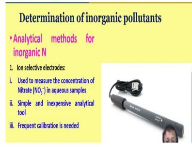
Now this ion selective electrode is used to measure the concentration of nitrate in aqueous samples and it is simple and inexpensive analytical tool. However, it requires frequent calibration. As I have mentioned that calibration is very, very necessary before you go for any analysis, so similarly in this case also frequent calibration is needed for this ion selective electrode.
