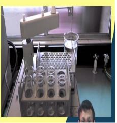
Now apart from these instruments also, there is an attachment called autosampler. Now, this autosampler is basically an attachment for automated measurements. Now automated measurements are easy to implement in soil analysis nowadays and most measuring instruments are equipped with the automatic sampling system. As you can see here, it is an autosampler of atomic absorption spectrophotometer.
