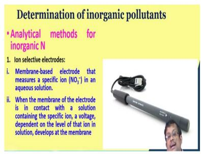
Now we are going to discuss about the analytical methods for inorganic nitrogen. The first tool which we generally use for determination of inorganic nitrogen in a particular ion is ion selective electrodes. Now, these ion selective electrodes are basically membrane-based electrode that measure a specific ion, for example nitrate in an aqueous solution.
