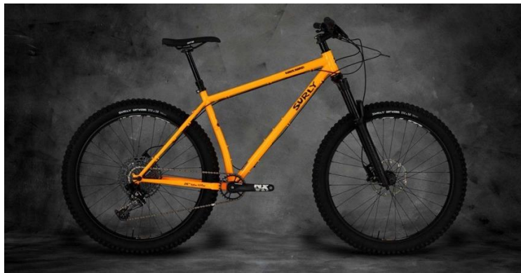
Figure 3 : a bicycle with two-dimensional truss
