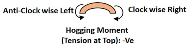
Figure 8 Sign convention of hogging moment
