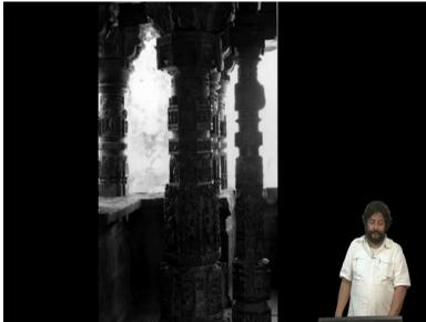
And the rounded bases are because the column has to be sliding later and it can only happen when the base is rounded at the bottom.
