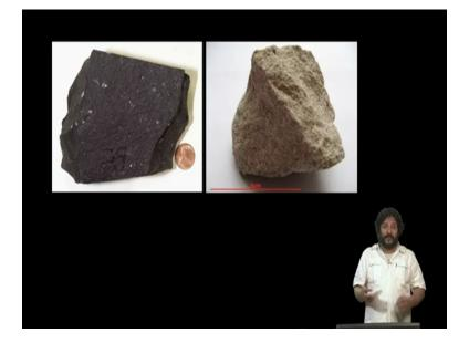
Now why is it that the temple fails all the four lintels crack and all of them have to be propped up by the stone columns? It is possibly because you have two different types of stone being used in Maharashtra and Gujarat. As we said, Anwa is in the basalt heartland and you have this dark black stone called basalt which has properties different from the sand stone that you find in Gujarat.
