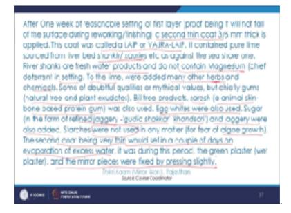
So, after one week of reasonable setting of first layer a second thing coat of 3 to 6 mm is applied this coat was called LAIP or VAJRA-LAIP. It contains pure line source from riverbed *shank* and *kauries* as against the sea shore one.
