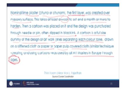
So, nominal lime plaster which is called is *Chuna* or *Chunam*, here what happens the first layer it was created over a masonry surface, this takes at least a week to set and a month or more to harden then a cartoon was placed on it and the design was punctuated through needle or pin.
