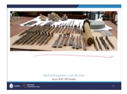
This is the entire palette, we also see the different kinds of tools within one family and how the dimensions change and lot of them are used for different purposes. So, sometimes on the surface, and sometimes when one has to go deep into the surface and do more detailing than another tool with another dimension is used. So, all those kinds of palettes
