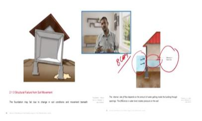
Then, when the water keeps coming into these areas obviously, there is also an aspect of; there is a difference in water levels for instance, the amount of water it enters and the amount of water outside, this is almost 8 cars, you know the load which is coming of the 8 cars worth of load which is pushing this wall and this difference in water level you know creates the pressure on the wall you know, this difference is creating the pressure.
