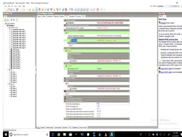
Along with this, we can have the mechanical ventilation, heating and cooling is definitely on when we are talking about air conditioning. We are talking about mechanical ventilation; we can also have the definitions for introducing the outside air. It could be per person or per area or it could be the sum per area per person plus per area.
