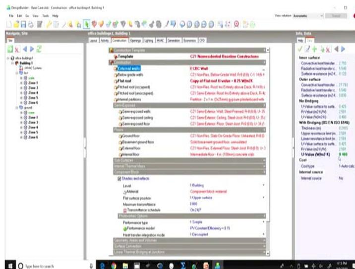
So, I have already shown you the process and I for your reference, I have changed the walls to ECBC wall, where the U-value, you can quick check it the U-value has been set as 0.4 which is prescribed in ECBC. I have taken the copy of a flat roof U-value, where the U-value has been prescribed to 0.33 which is as per the ECBC again.
