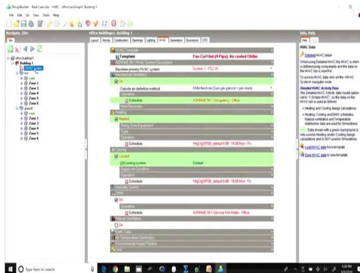
The next is HVAC; when we are talking about HVAC, automatically it has taken the template and the baseline primary system here will be taken as system 3 as per the ASHRAE.
