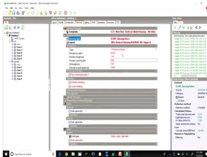
And in the openings I have changed the glazing type to ECBC glazing fenestration and if you look at the values here, I have changed it to U-value of 3.3 and a solar heat gain value SHGC value of 0.27. So, and keeping the WWR as 40 percent.
