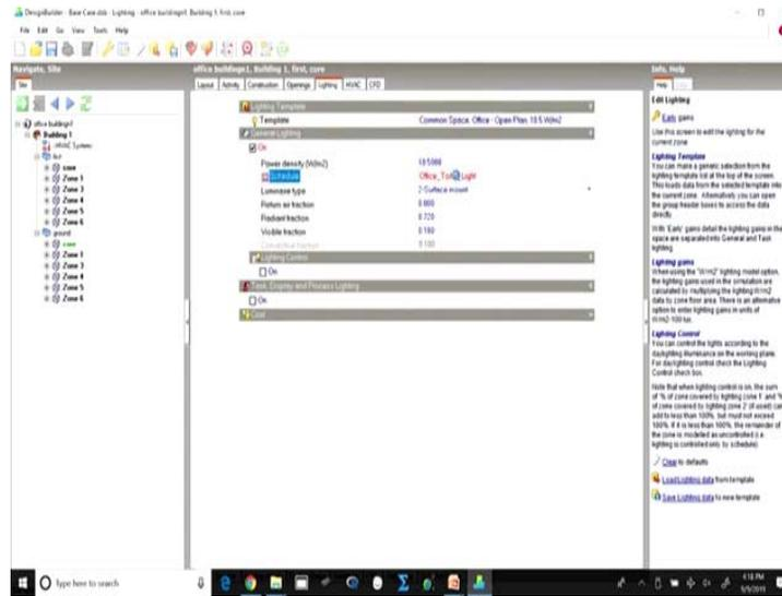
Let us check the core. So, for the core also, it is the same template and it is taken as 10.5 Watt per meter square which is what is taken even in the office toilet. So, the schedule although varies.
