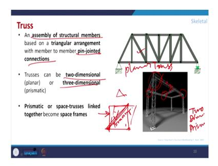
Now, come to the skeleton. So, this is a very useful you know component under that that is the truss. So, truss is basically assembly of structural members, ok. So they are joint together and mostly they are joint together with a pin joint, and this is to be formed in a triangulation form. Because, to start with suppose we have a portal like this where they are fixed, so on applied load what happened that it will try to you know get a deformation.
