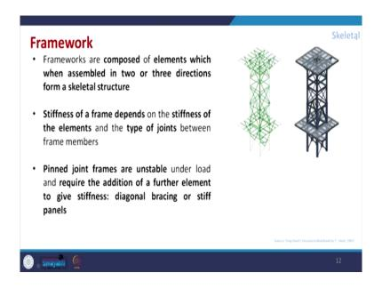
Now, come to the framework. So, here again it is a composed of materials which assembled in two or three directions. So, we just try to make a box, so it may be something like we just connect this part and then this part or maybe they are connected to give more rigidity, more stability with this bracing.
