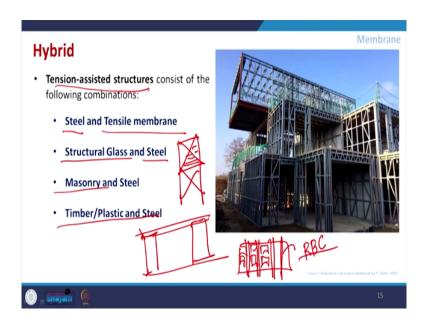
So, in that there are probably you know compositions like what we can call the tension as his structures. So, this is basically it may be a steel or tensile members. So, only steel being used as like post beam and then the cable is being used to add some membrane kind of structure to it. Then you may have the structural glass and steel as a combination. Here you can see what exactly like it is being still being used with other.
