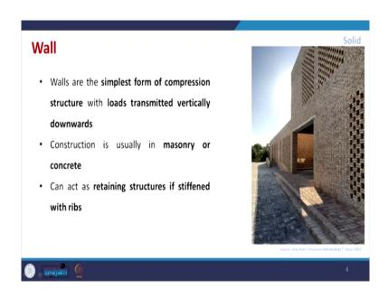
So, in this wall are the simplest you know form and basically it is the compressive structure and the way they will transmit the load is basically you know towards the gravity. So, whenever we create any building and also finally, whatever load imposed on it we will transmit
