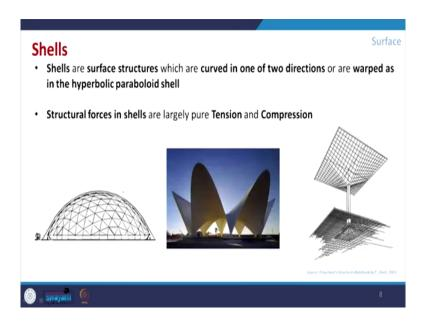
Come to the other surface category when again the thickness of you know that particular form is so negligible compared to the span it can cover. So, shell or the surface structure which had curved in one or two direction, so like it is may be of say something we just bend a piece of paper in one direction like this, ok. If I draw it correctly, so something like this.
