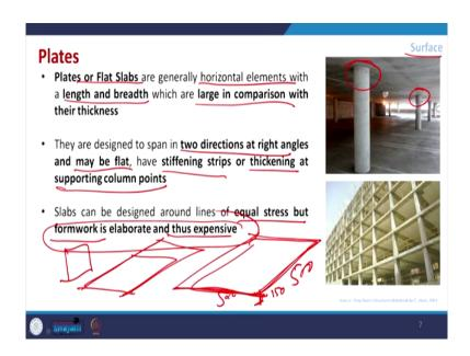
Come to the second example a under the surface where it is basically showing about what we discussed earlier also that is your post slab connection. So, you can see that there is no such beam or something just you the slab is resting on the post or column. So, plates or flats slab
