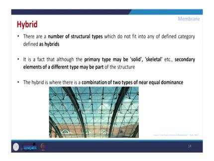
Now, come to the hybrid structure. So, we in this the hybrid structure basically where the number of structural types do not fit in the category that membrane or the (Refer Time: 24:05) like we said solid or the skeletal. So, that is coming into the hybrid category.
