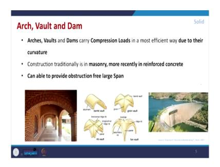
Come to the arch fault and dam again arch is again a very useful like what we can say the compressive structure where due to its curvature it transfer the load. So, load is very well transferred and because of the symmetricity, symmetry of this arch it will transfer the load to the you know the supporting column and then it transmit the load.
