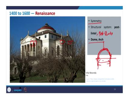
Come to the Renaissance period here with the symmetry played a role and almost you can see those style like, here also ionic column being used and it is similar to the Roman and all, but again it is your post lintel and your post slab structure, along with that the central dome arches being used.
