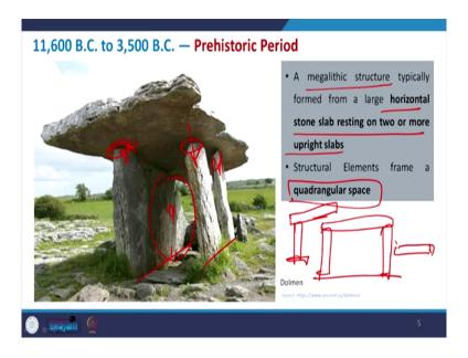
This is another example of dolmen. So this is basically the megalithic structure. So, megalithic structure is basically where you know horizontal you know slab is resting on the upstanding slab. So, if you take a particular slab like stone slab and then you make it you know upright in this position and you put another one again no mortar being used. So, you can see that how it is resting there.
