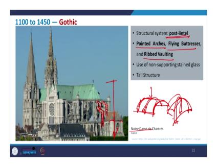
Now come to Gothic, Gothic era is specially known for its ornamentation of structures. So, basically here you see the basic structural is again your post lintel and post slab also and then you can see that pointed arches then flying buttresses and ripped vaulting these are features of this.
