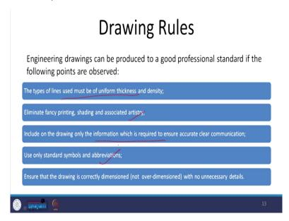
So, one that the lines that will be used they have to be of uniform thickness and density. When we move the pencil so things have been made much simpler with the help of these CAD software, computer aided drawing software for example this AutoCAD is there, you have many other software which are used to draw these drawings. So, it is much easier, you select a line thickness and you draw a line of a certain dimensions, certain measurement.
