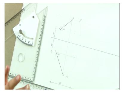
So, say we again have a line which has a length of 8 centimeters. Now it is making an angle of 30 degree with HP and an angle of 45 degree with VP and nearer point to reference line is 3 centimeter above HP and 4 centimeter in front of VP. This is what the given condition is. Let us see how do we draw the final projections of this line which is inclined to both the planes.
