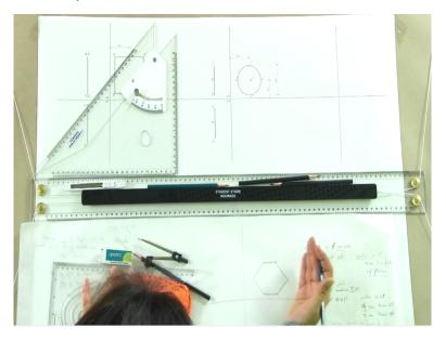
So, let us start with first problem where we have say a square of 8 centimeter side or say 6 centimeter side which is perpendicular to both HP and VP and its center is at 4 centimeter from both reference planes. So, we have a square plane which is perpendicular to both HP and VP and its center is at 4 centimeter from both the reference planes. Now to start with I have already drawn these VP, HP and a side plane here.
