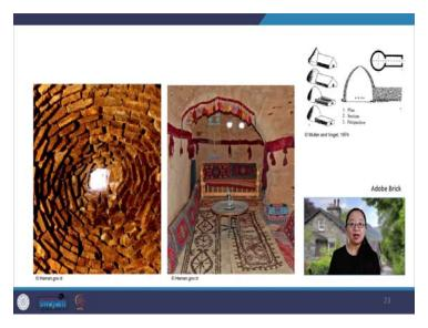
These houses resist the stresses of strong winds and minor shocks from frequent earthquakes since the mid-18th century. The doors and windows are few and small to minimize the Sun's glare and the movement of hot and cold air during the day and night. Its floor slightly raised above the soil outside spotlessly clean with a recess for cooking and attractive decorations in bright tensile paper on the walls.
