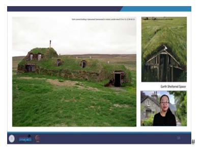
The third technique is the earth sheltered space. It is a traditional technique, but nowadays commonly referred to as green roof. For 1000s of years in arid climate earth has been traditionally used to cover roofs, it acts as a thermal mass regulating the inside temperature. Earth material absorbs heat and retains it before gradually releasing it into its surrounding.
