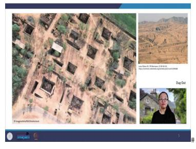
The first construction to be discussed here is that our technique which falls into the monolithic construction, where one use only the soil, Earth is dug out of the ground to create underground shelter. In most cases, this kind of dwelling occurs in zones with arid climate, and with soft and easy yellow Earth to dig into, but also has a high capacity to maintain the standing posture and less prone to collapse even without support.
