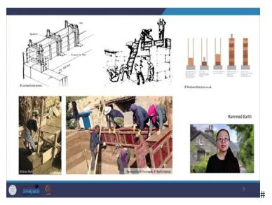
The second one is Rammed Earth technique, which also belongs to monolithic construction. This technique is basically making use of simple tools to compact soil in order to produce rock-hard structure. The construction of rammed earth includes aggregate portions of silt, sand and clay and adding this mixture to the soil.
