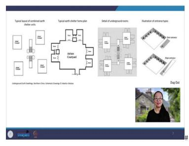
The dwellings are dug 6 to 10 meters deep for the sunken courtyard. A ram is also cut into the sides of the courtyard to allow residents to move easily from their homes to the ground level above. Then the rooms are carved out from the four walls of the sunken courtyard, the interior of the rooms may also be reinforced with stone and clay walls or columns.
