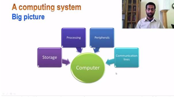
Let's start by looking at general structure of a computer. A computer consists of four major elements, major components. One is storage. Another is a processing element or the CPU. You may have peripherals such as a camera, a keyboard or a monitor, and then it may have a communication interface, which allows this computer to be connected to a network, for example, the Internet.
