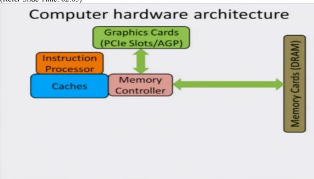
Additionally today in the computers you will find graphics cards for carrying out rendering of scenes and also for doing high-performance computing. These cars are normally connected to the memory controller through a special kind of fast buses that's called a PCI Express bus.
