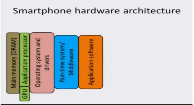
Between the application software and the application processor sit two elements one is the operating system and the drivers that are necessary for handling various types of I/O calls. We'll look at the I/O devices very soon and a runtime system or the middle layer which the application software takes help off to execute various types of application programs. (Refer Slide Time: 01:22)
