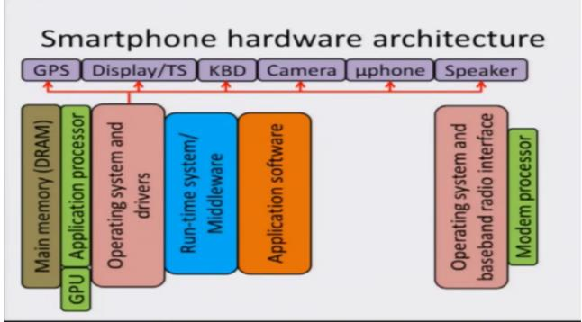
The communication is handled by a modem processor which receives all the signals and passes them on to the operating system and the baseband radio interface. (Refer Slide Time: 01:46)
