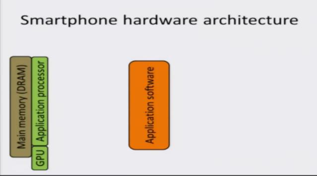
The software gets executed with the help of an application processor often taking help from a graphics processor for rendering scenes and whenever the application processor of the graphics processor needs data it will access the main memory which is dynamic random-access memory.
