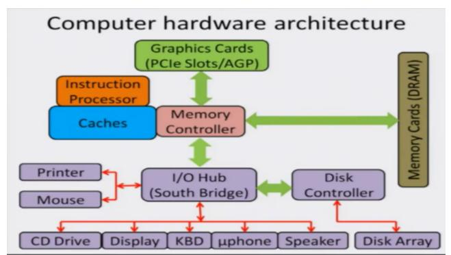
Additionally the south which connects to several other I/O devices, for example, the printer, the mouse the CD-Rom drive, the display or the monitor that you see, keyboard, microphone and the speaker. So this is roughly the overview of the motherboard which plays a key role in how a computer works. Thank you.
