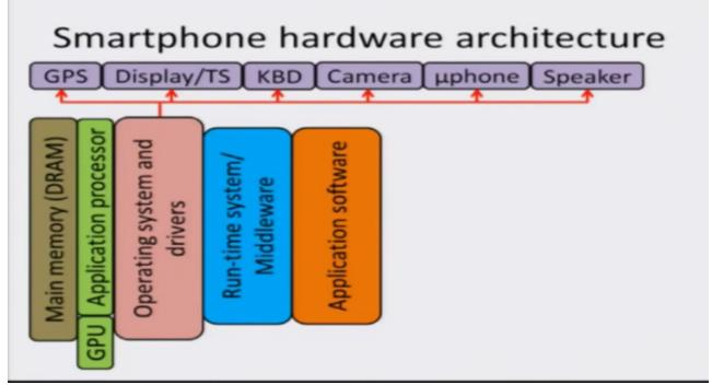
The operating system must have drivers for various types of peripheral or I/O devices for example the Global Positioning System, Display and the Touchscreen, Keyboard, Camera, Microphone, Speaker and so on. (Refer Slide Time: 01:35)
