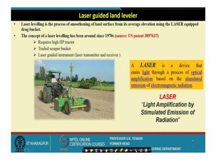
What is a laser guided land leveler? Well we see that when we want to know the topography of a particular field, we have the civil engineering methods by which we do we use the del p level and all that, and we find out what is the elevation and depression of the different locations in the field.
