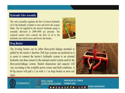
Yes, here is the hydraulic valve assembly here. The valve assembly regulates the flow of tractor hydraulic oil. Now generally in a hydraulic system what is there. In a hydraulic system we had certain components. For example, there will be a location where there is hydraulic oil.
