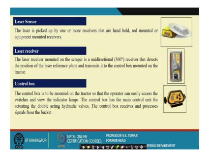
The laser sensor;tThe well the laser is picked up by one or more receivers, that are handheld rod mounted or equipment mounted receivers. Now this laser receiver is
