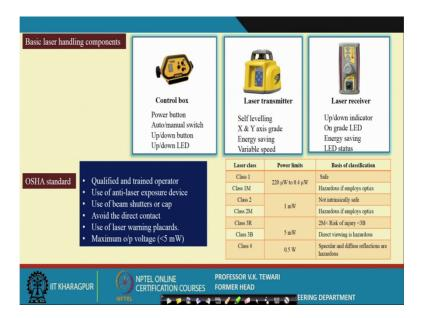
Levelling, laser land handling components; detailed components which we saw there; the control box, the laser emitter transmitter, the laser receiver. So, transmitter receiver and the control box very important one. Because one transmits the other receives and then gets back to the control box which will do the various operations.
