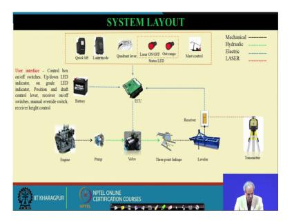
The system layout a greater, system layout is shown here you can see that the user interface the control box on off, switch up down led indicator or grade led indicator position, and draft control lever receiver on and off switches, manual override switches receiver height control.
