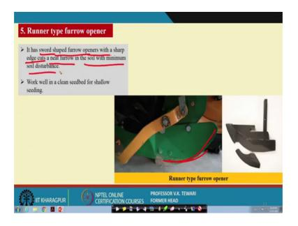
Runner type furrow openers well runner type I have shown you already that this is you used on a pneumatic seed drills you can say furrow is. So, sword shape furrow just like you see, you can see that this is a sword virtually sword furrow with a sharp edge cuts a neat furrow, in the soil with minimum soil disturbance this is what it does these are generally used in generally we have shown in the such devices being used in pneumatic seeders.
