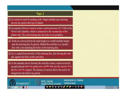
In type 2, a suction is used pic for picking the seeds. We would like to start from a in a drum where, the seeds rotate where the a drum is rotating and the suction pressure suction is created, a vacuum is created in a drum. And, that the device this is singular modular type metering devices are used in this type of planter.
