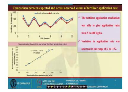
Well when we compare this with the output the results of these two we find that we are not very much off, the fertilizer application system we find that we are in a position to give application rates between these two vary as low as 5 to about 400 kg; that means, for a smaller seeds also we can do and as high as high application rate and the variation in the application rate is not very much, it is very small.
