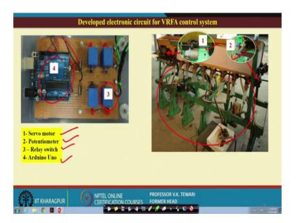
Well developed electronic circuit we can show that here the just the Servo motor, the Potentiometer, Relay switch and Arduino Uno all these are shown over here; 1 is the servo motor here, 2 is the potentiometer in this case, the 3 here is a relay switch and 4th is the Arduino Uno. So, we are in a position to show you and this is the unit which has been developed in the field and in fact, we have operated and this has given us a result which is very close to our acceptability.
