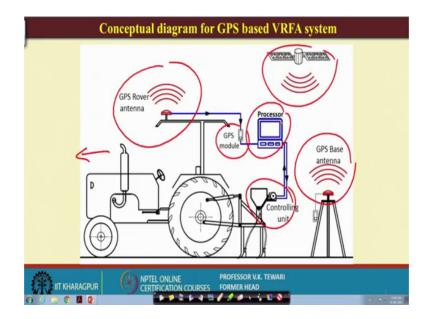
Now, this is the conceptual diagram of a GPS based system here, you can see. This is the GPS rover here then this is the satellite here information the GPS antenna base which will be there outside and then the processor, the GPS module in this and then here is the controlling unit and this is the location which we are going to apply.
