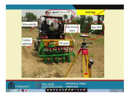
Well, field test we have done field test of this let me have a look at this. The micro controller, the micro controller is here, the fertilizer applicator is here. Then these the DC motor at this location and the roller position sensor roller position sensor ok, then base GPS is here, rover GPS is in this place.
