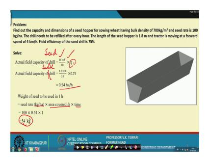
Now, problem has been given to you. So, that you are in a position to understand what is this and how do we how do we actually use information or knowledge which has been given to you it is like this. Find out the capacity and dimensions of a seed hopper for sowing wheat having bulk density of 700 kg per metre cube and seed rate is 100 kg per hectare, the drill needs to be refilled after every hour this is the requirement.
