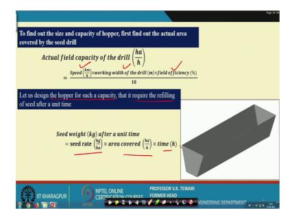
Find out the size and capacity of the hopper, by well to actual area covered by the seed drill.
