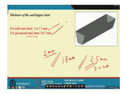
Thickness of the seed hopper well; considering all machine design knowledge and the total weight which is coming onto the hopper material and the shape etcetera, I am sure you would be in a position to find out what is the thickness and you will go to the market for selection of that that materials thickness and many a times, if you see that the see you find out the thickness is about 2 mm and the sheet which is available either for 1.8 mm or mm or is available for 2.5 mm or 3 mm.
