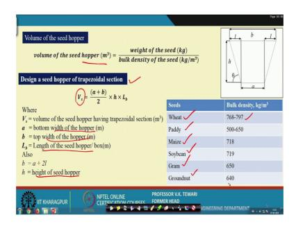
So, the volume of the seed hopper now then it is easier now it its very simple if you go through the details of this diagram which I have given here, we will be able to understand how to get the volume of the seed hopper.
