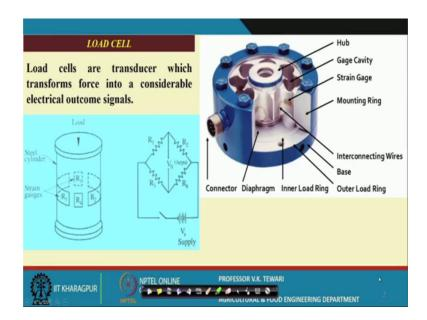
It is very essential as well to also know about what is this load cell and all that just this information we have gathered from literature, so that you can you can appreciate this point of what this load cell is in fact. So, this load cell load cells are transducers which transforms force into a considerable electrical output signal. Now, this is what, it is what
