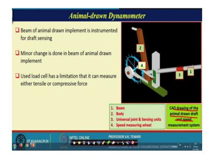
See, the while we developed this we also wanted that how do you measure these draft for animal drawn equipment. It is worth knowing animal drawn equipment and even the one which we are talking with respect to the manual drawn as well. So, in animal drawn equipment where do we keep these dynamometer and for that also we have used a similar concept. This is the CAD, CAD drawing of the animal drawn draft and a speed equipment here.
