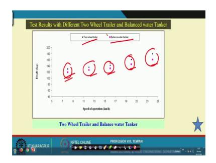
Well, here two results with two different two wheel trailers and balance will tankers. Now, this they result only to explain to you that the draft values which are two wheel trailer and balanced water tanker. You can see the differences are not much we. We can say here that we are very much accurate in both the wheels by which we have measured the two wheel trailer and balanced water tanker.
