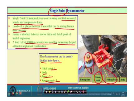
Single point dynamometer. Well, this is also important because some we test through the tractor not only the implements or equipment, but we attach also the haulage equipment which is mostly the trails the water bowsers or the trailers in which we carry lot of haulage material you can say you can think of either it is the and the bio-product oh or the actual material like paddy wheat grain or the straw etcetera, which are being carried.
