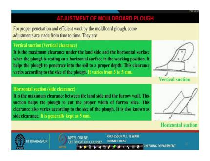
These are two very important adjustments sometimes when I want to increase the depth then the adjustment is vertical section which is over here.
