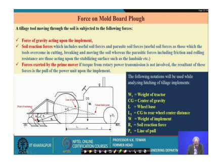
Forces on mold board plough well we have shown already these forces on mold board plough, generally as I showed that force of gravity or the implement which is there, the weight of the implement and the soil reaction forces and the forces exerted by the prime member in case of a rotary power source is the power rotary power source is not involved, the resultant of these forces is the pull or the power unit upon the implement.
