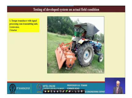
In the field, well, this is a developed system on actual field condition. This is how it works in the field condition. Well, you will see the operation of this field testing of this unit. You can see that how here the this unit is in the operation condition.
