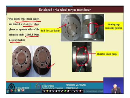
The how the concept has been developed I am giving you the secret behind this. In fact, how did we do this? See, this was developed in fact, we have made flanges and these flanges will be on the tractor wheel on one side and the other will be with the axle. So, the extension will take place with this.
