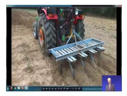
Now, you can see an arrangement to with the respect to cultivator. You can see a cultivator being used in the field and we are in a position to measure this. Now, this is to show you that all these equipment can be used and then we can have these information collected by using the instrumented tractor.
