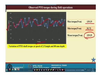
Observe PTO torque during field. Yes, what did you get the during this field testing, what did you get? We saw that we have got values in the maximum torque we got here for a particular equipment which was connected and then the minimum torque was this and the mean torque values are this. Now, these you can see here that the variations which are shown over here these are the actual things with respect to time then the PTO torque Newton meter measurement here.
