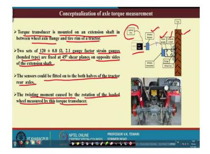
Conceptually conceptualization of the axle torque measurement. How do we conceptualize this; that means, where do we keep or where do we measure? Because you see the tractor axle you have seen the tractor axle, it is very difficult to approach in the tractor axle. You very difficult to locate at the place where we should put, but there is no space for that. So, first of all you need to get any space where you will have this. So, what is the concept behind this let us have a look at this.
