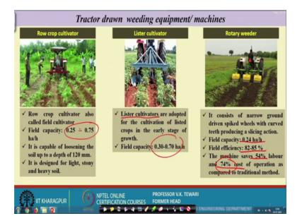
Now, these are the tractor drawn units. Well, tractor drawn units various types of tractor drawn units have been used by different locations and you can see that what are their names etcetera you can see row crop cultivator. See between the rows how this tractor drawn unit is going and it is cleaning this very nicely. It is earthling up doing earthling up because you create some sort of a when you do this cleaning of the weeds you also create remove the hard crust after three weeks of operation.
