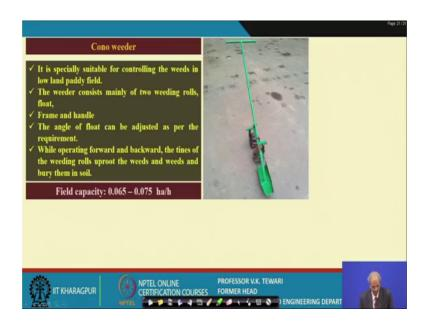
Cono weeder. Well, this is a device which is generally used for lowland conditions because particularly for paddy. So, you will see that for paddy we use this thing and since these also a push-pull type of device, but then it has the two different types of cutters or the cutting element which is there.
