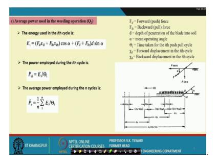
Well, average power used in the weeding operation, what is the average power used well if you talk of the cycles, we have talked of various cycles when we saw in this that various cycles have been used, from cycle i is equal to 1 to i is equal to n. Then average power used in the weeding operation will be then you the average power here will be yeah, this is the X if talks of the forward in the distance displacement and F if we talk of the forward force applied.
