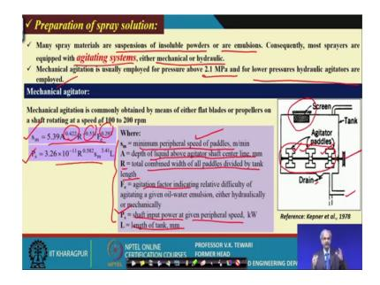
Preparation of spray solution, how do you prepare this spray solution? This is important, sometimes you have the emulsion which are oil emulsion liquids which are which need a constant stirring, otherwise the solution will not remain colloidal throughout on the process, and otherwise when you want to apply you will find that the chemical is not actually in the same concentration which it should be there.
