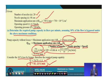
Let us see how do we approach the first is determine the required pump capacity. So, what is given here in that see the nozzles as I said we have been given to you the nozzle spacing is also given to you. Then maximum application rate is 750 liter per minute is given here. Now, this you can, because you want to change it to hectare or per square meter you want to check this you can see this. Then operating speed is 6.5 kilo meter per hour. Operating pressure, which is also given 520 kilopascal.
