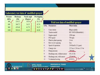
Now, we wanted to compare certain values with respect to this here; Laboratory test data and Modified sprayer here Field test data of modified sprayer here. So, in the laboratory what we got? See. This is important because the until unless you test this under laboratory and the field conditions you may not be in a position to appreciate what we have got.
