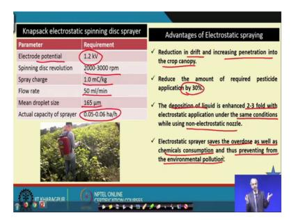
Knapsack (Refer Time: 26:29) spraying disc now. Advantages we see here, we wanted to explain to you the knapsack electrostatic spinning disc and the advantage of electrostatic spraying. Now, this is worth showing you here because then you will understand what are the advantages, which we get through a particular unit and what we do not get.
