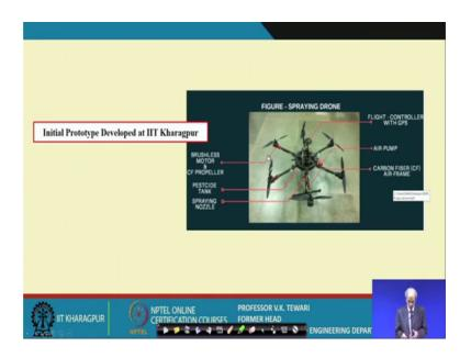
Initial prototype development as so, we developed at IIT Kharagpur, we developed a small prototype about 500 gram payloader (Refer Time: 17:34). And we would like to show you this the working of this here, the details are you can have the details here in the system.
