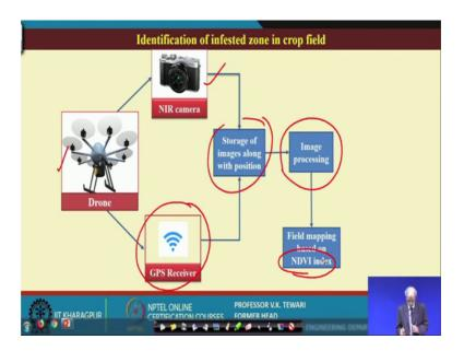
Identification of infested zone in a crop field; now, how will you do this, see this particular concept is given here to understand. You have the drone here, you have the drone here. Now, the NIR camera is here, storage of images along with position, now you need to store the images. The processing of the images have to be done.
