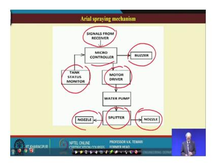
Aerial spraying mechanism; what is this aerial spraying mechanism? Well, if the same thing has been put it slightly in another way, the see the micro controller see the signals from the receiver, see microcontroller, then the tank of the status monitoring microcontroller.
