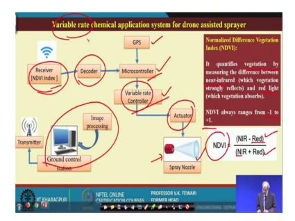
The variable rate chemical application system for drone assisted sprayer. Now, the whole thing has been put here again, now you just see how these some more details are there. You can see here the GPS, fine; you have the microcontroller, yes; and the variable rate controller, it will like to control this.
