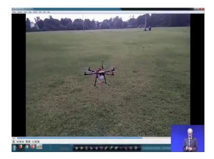
Now you can see that this is very small one about five 500 grams payload capacity, we will just tested, because the aim is to make a small is possible, which will be in a position for the farmers small farmers, who can use this. Here is spraying and showing you whether there is spray can (Refer Time: 18:44) you can see the spray which is coming out of this, this is being controlled. And the distance you can vary above the ground as well as the in the horizontal direction.
