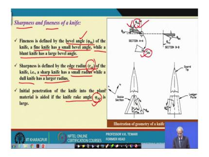
Well, sharpness and fineness of a knife, what are these important parameters actually, these are very important parameters. The sharpness of the blade is important, how fine is that blade sharpness. Now, here fineness is defined as the bevel angle so, this bevel angle b phi bk, this talks of the fineness of that a fine knife has a small bevel angle, while a blunt knife as a large bevel angle.
