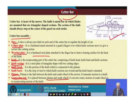
This is the cutter bar so, in the cutter bar, there is important things which are here in this cutter bar, which has been shown here the in one of the sections of that from the side. And what are the details of this, you can see the cutter bar assembly as the shoe the ledger plate, which you have talked of. The wearing plates, which are there, hardened steel material, then knife is there, and knife section will be there.
