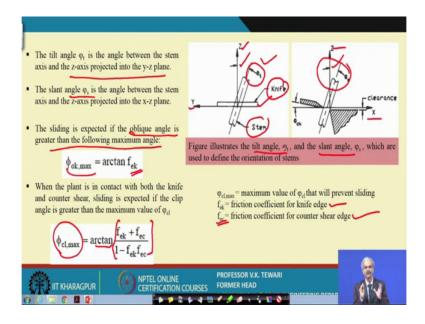
Well, how the whole thing takes place, when the plant is cut. Now, you have a look at this then so, the tilt angle is the angle between the stem and the z-axis is y-z now. Here see this is y-z plane; this is z, this is y so, in the y-z plane, this is tilt angle, this tilt angle here. So, it is important about when this is the knife, which is cutting, and this is the stem, this is a knife here and this is the stem, which is written here, you can have a look at it.
