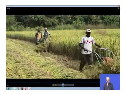
I have a look at the video how it works? You can see how it works here. Actually see the windrowing is going on properly as we have set. And if you can see there are 2 machines being operated, so the working is faster. They very fast they can cut these you can see here that the 2 persons are operating. And they have been used effectively for so long. Now, the other what is your problem with these is that they are just windrowing now there are devices where only windrowing will not do.
