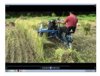
So, we will have a look at this actually how the whole thing is being perform. You can see the bundles being made see the bundles which are being made here. If see the back from this side the bundles are being, so it is easier for the farmer to collect these bundles and then transport.
