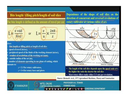
Now, we just talked of the length of the soil slice. Now how important is this length of soil slice? See definitely important because then we would know as to what is the total volume of soil which this rotavator is handling, because on that itself the power will depend and we will have to have the power source accordingly designed.
