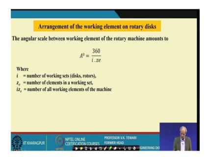
Now, these are arranged with respect to see the space you give here regular space is A 360 by i into z into e here. There is number of element working elements and number of working sets. So, once we know that because 360 is the rotation of that. So, we should be in a position to find out the value A which is the working element angular scale between the working elements; that means, angular positioning of the between these two.
