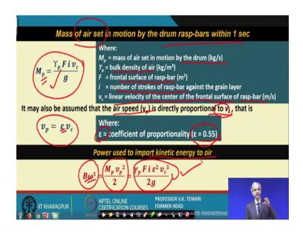
Mass of air set in motion by the drum rasp bars within 1 second or per second because we would like to know: what is the mass of air set in motion. See what happens when the drum is rotating there will be an air which will be also moving along with that. So, what is the mass of air which is put in motion when the drum is rotating and that when you have the concave. So, this air is coming inside when the material is thrown inside the concave between the drum and this.
