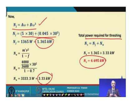
So, you can just if you put these values, you can see here that N j the force and which is talking of the idle resistance can we find out from putting all these details and this is the value of N j which is. So, 1.365 kilo watt possibly this is higher value than when you are talking of a bigger one, you may find that this is the ideal resistance which is required; if you talk of the total and then is useful one which talk; so, this.
