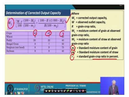
Determination of corrected output capacity: well this is another important parameter which must be done. This correction particularly with respect to the moisture content, and the grain crop ratio; this is particularly with respect to that you can see here that m 1, m 2 talks talk of the moisture content of grain at observed grain crop ratio, moisture content of the straw at observed grain crop ration of grain and straw
