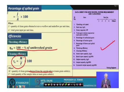
Percentage of the spilled grain: quantity of clean grain obtained at sieve overflow and underflow per unit time. As if you know the total grain input and how much is this spilled grain you were talking of that means, how much is the clean grain obtained, so the ratio of that will give you percentage of spilled grain. Similarly now, when we talk of threshing efficiency, now threshing efficiency here 100 minus percent of unthreshed grain.
