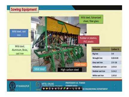
Let us go to Sowing Equipment you we have talked of this sowing equipment earlier and more details are known to you know about all the components which are there in the equipment which starts from the hopper and then goes to the tines and then it goes to the tube. Then it has the mitring shaft mitre mechanism that the power transmission etcetera.
