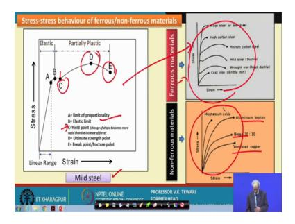
Now, so, we wanted to wanted to give you since we have talked of the materials it is worth and very logical and very imperative, that we also talking about these stress behaviour of the ferrous and nonferrous materials. Now in case of mild steel which is the one, which is very widely used in all the equipment that we have talked up so far.
