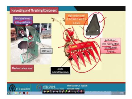
Well Harvesting and Threshing Equipment, we are talked of this equipment already and we know the various components of these equipment, see the mild steel. Now I have given you here some of the equipment which we have and we would like to you to have a note of this. That is why it is worth understanding that instead of telling you that this is made of this and that we have the equipment here and we wish that you take a note of these.
