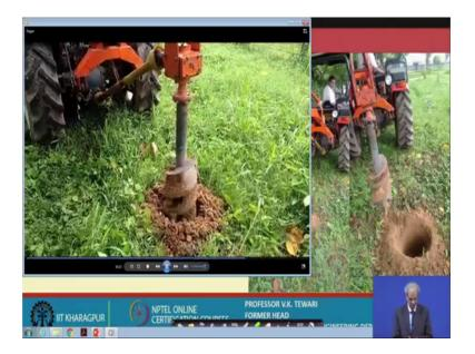
See let us see yeah you can have a look at this how it is connected you can see that this connected to this side from here and then this is the auger. Now, we will see how this operates the power will come to the PTO through this Cardan shaft and then from here to this box here. And then it will come to this yes you see the operation here you can use it anywhere you want.
