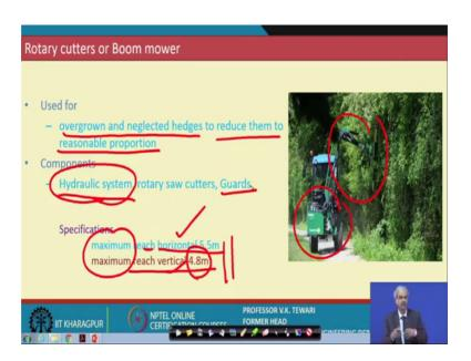
The rotary cutters or boom mowers sometimes we are we would like that the whole tree sometimes streaming of the trees are required. And maybe it is not possible that people can go on top of this and then trim it, but then these machines are available and these machines can do the job of trimming.
