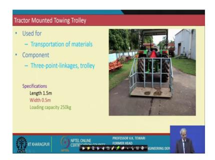
Now, another tractor mounted towing trolley this way we have developed at IIT Kharagpur in fact, it is not a big job done. But then this is the one which we are using it and for you can see that in a small area in a small locations if you want to have you can use this thing.
