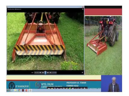
So, you can have you can see that this you see here that Cardan shaft is rotating taking power from the PTO there and this is the hole slasher, here below this we have the blades which are there two blades are there in this. And the rotary blades which are there and at the end the blades are connected we will see the operation of this when it will starts moving yes it is started moving.
