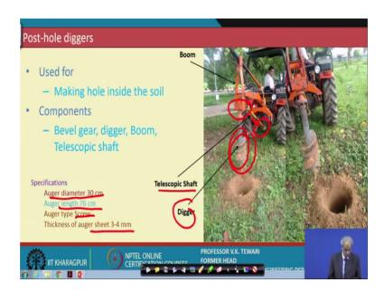
Well another thing which I said earlier is the post hole digger this is one equipment which is very extensively used in most of the operations particularly for orchards development and different types of plantations which we want to have.
