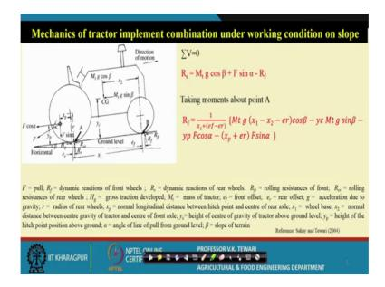
So, here we have said that there is a force here. And this will have 2 components very simple as you have seen earlier that when there will be a line of pull, through the line of pull there will be a pull force acting. So, the horizontal component will be the pull, and this P y will be acting downwards. Now this is the location where it acts where the weight of the implement is also acting at this particular point
