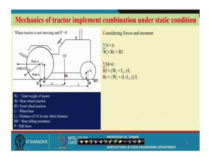
Yes, mechanics have tried to implement combination under static condition; where you must have seen that when the tractor is simply standing condition, and when the this P is
