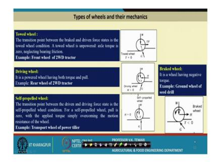
There are certain other aspects which need to be explained about the wheels. See wheel a simple wheel which has only to be pulled here, we call this wheel where there is no no torque this torque is not there. So, this is towed wheel.
