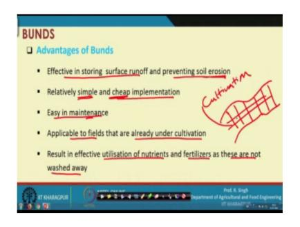
Some of the functions we have already seen. So, advantages are related to that, they are effective in storing surface runoff and preventing soil erosion. We have already seen in great detail that in between 2 bund sections, the surface runoff whatever rainfall is occurring that gets stored. And obviously, because the flow of water is not taking place; so, the soil transportation is not taking place; that means soil erosion is prevented.
