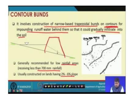
Then just to give you an idea about the two types of bunds we talked about that is contour bund and graded bund; which we will discuss in great detail later on. So, basically contour bund involves construction of narrow based trapezoidal bunds on contours for impounding runoff water behind them. So, that it could gradually infiltrate into the soil.
