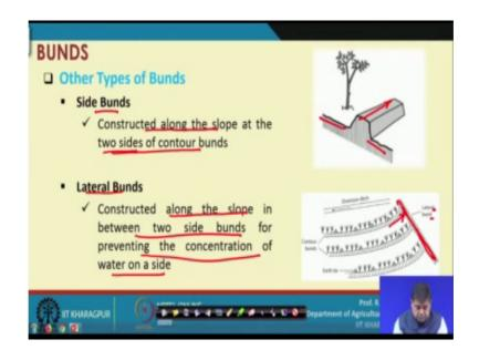
Then there are some other types of bunds associated bunds also. For example, side bunds. The side bunds are constructed along the slope at the two sides of contour bunds. So, this is across the slope and along the slope just on this side of the contour bund. We construct these bunds which are referred to as side bunds; because they are built on the side.
