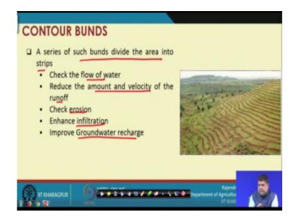
And the functions are the advantages whatever we say we have already seen. Series of such bunds divide the area into strips which we have already seen. Check the flow of water, reduce the amount and velocity of runoff, they check erosion they enhance infiltration and improve groundwater recharge. So, very similar already we have discussed the functions of a bunds. And these functions of contour bunds also are more or less in similar lines.
