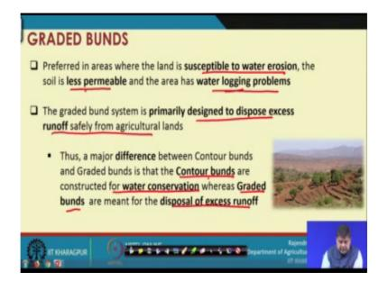
And these are preferred in the areas where land is susceptible to water. Erosion soil is less permeable and water logging problems are there so; obviously, soil is less permeable. So that means, if we stand for longer period time infiltration will not place take place and water logging will take place and that is why we go for graded bunds and primarily designed to dispose excess runoff safely from agricultural land. So, that is the main function.
