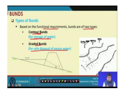
Now coming to types of bunds; bunds are of based on the functional requirements bunds could be of two types that is contour bunds, which are used for storage of water, and graded bunds which are primarily used for safe disposal of excess water. So, two category of bunds are used, similar kind of structure we will go into details of these in the following lectures.
