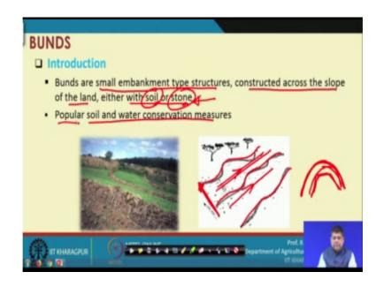
To start with the bunds; bunds are basically a small embankments, embankment type structures constructed across the slope of the land either with soil or stone. So, their important components are: they are small embankment type of structures; that means, simply kind of embankment or dam what you see, that is some kind of a cross section some like this or whatever be the section this is how they will look like.
