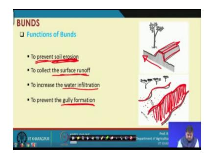
Now, coming to functions of bunds; the functions are, that is they are built to prevent soil erosion, to collect surface runoff, to increase water infiltration and to prevent gully formation. As we have already seen we have seen that this is this is the typical cross section which we have seen which is a trapezoidal kind of cross section, which is shown in this picture.
