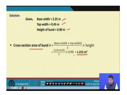
So now given the base width, top width and height of the bund the cross section area of bund can be easily calculated we know the, this is a trapezoidal section. So, the cross sectional area comes out to be 1.215 square meters and once cross sectional area is known.
