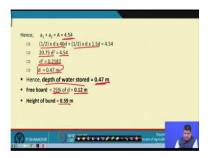
So, here a 1 plus a 2 has to be equal to 4.5 4. And a 1 a 1 and a 2 from these are nothing but simple triangles. So, basically in terms of d we can write half times d into 40 d and half times d into 1.5 d. And then by simplification it comes out to be 20.75 d square equal to 4.54 or d square equals to 0.2147 or d comes out to be 0.47.
