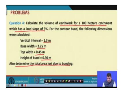
Now, let us take the last problem. That is a calculate the volume of earth work for a 100hectare catchment which has a land slope of 3 percent. The following dimensions are given the vertical interval is given base width is given top width is given, height of the bund is given and we have to also determine the total area lost due to bunding. So, let us say how to handle this problem.
