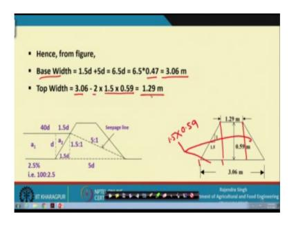
That is for stability, seepage line must pass through the base of the dam. And seepage line we defined that is the top fretic line is referred to as seepage line. And the slope is 5.5 is to 1. So obviously, this is the total base width which has 2 components this which is equal to 1.5 d, and this which is equal to 5 d that simply means that the total base width is 6.5 d and 6.5 d and because we know the value of d already 0.47 meters; that means, base width will be 3.06 meters.
