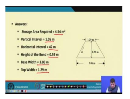
So, thus we can write that the total answer we can write that storage area required for 4.5154 meters. Vertical interval 1.05 meter, horizontal interval 42 meters, height of the bund 0.59 meters, base width 3.06 meters and top width of 1.29 meters. So, this is how we solve the problem.
