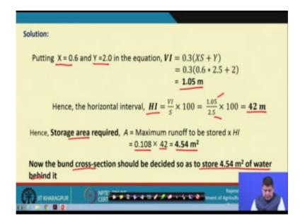
So now coming back to Ramser formula and putting x equals to 0.6 and y equals to 2 in the equation, we get vertical interval equals to 1.05 meters. And thus the horizontal interval which is VI by S into 100 where S is the land slope, by putting the values of VI and S given values one VI is already calculated S is given as 2.5. So, the value which we get is 42 meters
