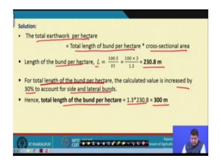
So, first thing we require to calculate the total earth work per hectare is the total length of bund per hectare times cross sectional area. Because that is the total earth work required. And length of bund per hectare is given by 100 S by VI or it comes out to be well putting the values of S and VI it comes out to be 238.5 meters
