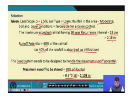
So, let us see that what are the data which are available and what we need to calculate. So, here the land slope is given as 2.5 percent. Soil type is loam, rainfall is moderate in the area, soil and cover conditions are favourable for erosion control. And maximum expected rainfall having 10 years recurrence interval is 18 centimetres or 0.18 meters.
