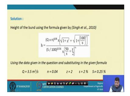
So in this case, we can straight away try to use the height of the bund formula which we saw we almost derived using such paper. So, is where h is a function of Q n z and 2 slopes capital S and small s remember capital S is the channel bed slope and S is the land slope. So, all the values are given Q equals given as 3.5 cubic meter per second. N is given as 0.04 and z is 2 S is 2 percent capital S is 0.25 percent. So, all the unknown values are given.
