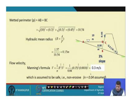
Now, next thing we have to calculate is wetted perimeters and wetted perimeter, we saw that it is nothing but the length that is in constant touch with water. In this case, it will be AB and BC. So, AB and BC we can again same triangle 2 triangles are there. So, we can find out AB square equals to BD square plus AD square that is 10 square plus 0.3 square.
