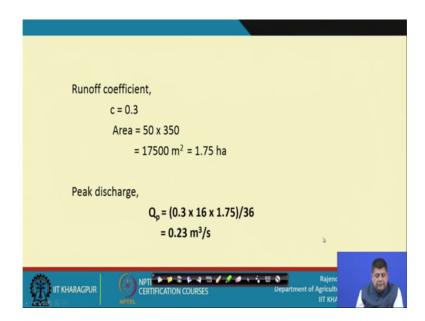
So, once TC is known we can the intensity is known we know the C, we know the total area because H HHI and L are known. So, area is known. So, we can put in rational formula to get the value of QP which comes out to be 0.23 cubic meter per second.
