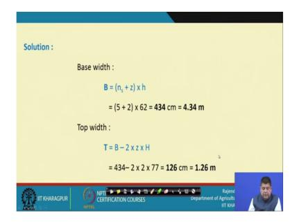
And once h is known, rest of the things are simple we know that bed width is depends on n S plus z equal to going to times h n S is given as 5 is to 1 that is the seepage line slope z is given as 2 is to 1 that is z is equal to 2 h. We have already calculated 62. And so, that comes out to be 4.34 meters.
