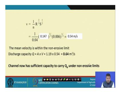
And then, we have to now calculate once again the velocity which is 0.54 fine still fine. And then Q value we have to calculate which comes out to be 0.64 square cubic meter per second, which is sufficient because the discharge we have to handle was 0.23. So, channel now has sufficient capacity to carry Q P under non erosive limits so; that means, we have handled the problem.
