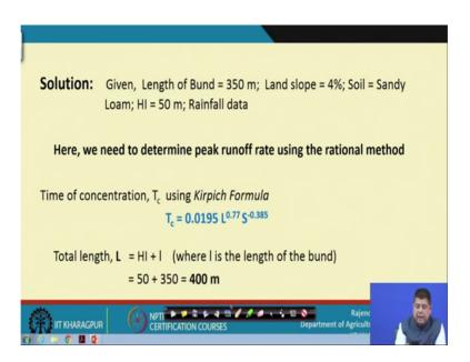
So, data available are length of bund 350 meters land slope 4 percent soil sandy loam H I 50 meters and rainfall data is given so; obviously, here again we have to determine the peak rate of runoff using the rational method in the previous case which we handle rational method. They are we had been given rainfall for time of concentration for duration equal to time of concentration, but this is not the case.
