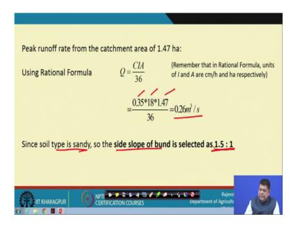
And once drainage area is known, then we can put the value in Q equals to CIA by 36. So, C is known 0.35, I is given as 18 centimetre per hour. The drainage area, we have already calculated is 1.47 hectares by 36. So, the value of Q comes out to be 0.26 cubic
