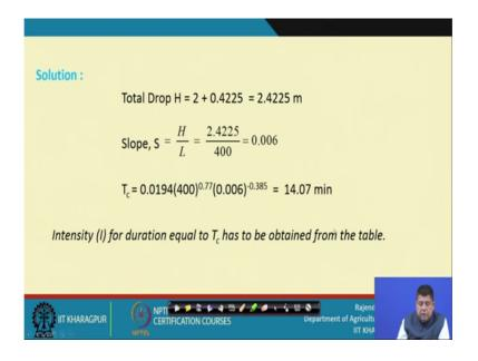
And thus the over the channel the total drop which comes out to be a 0.4225 meters and the total drop comes out to be 2 plus this that is 2.4225 meters and; that means, the total slope will be H by L. That is the total drop by over length this is drop this is length 0.06. So, in formula now we know L we know S. So, by putting this formula we get a value of 14.07 minutes. And then we have to use this for obtain the data from the table itself.
