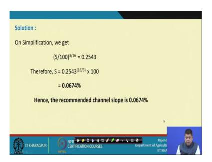
. That is the recommended channel slope is 0.0674 percent that is what we have to calculate we had to calculate in this particular problem.
