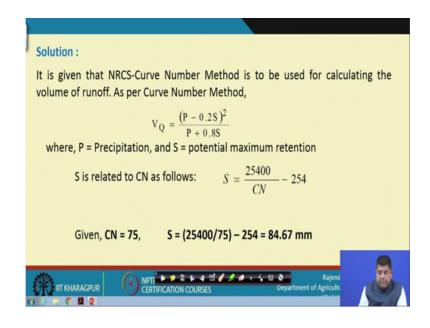
And if you remember the NRCS curve number method used for calculating the volume of runoff in depth units. And this is how the curve number looks formula looks like VQ equals to P, which is precipitation S which is potential maximum runoff and P minus 0.2S square by P plus 0.8S and S is related to curve number by this formula S is equal to 25400 by curve number minus 24, 254. This is when S is in millimetres, this particular formula is used.
