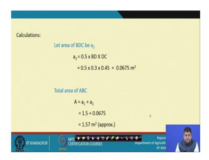
Ah BDC a 2 which is half into 0.345 into that is comes out to be 0.0675 square meters. So, total area of ABC is a 1plus a2 comes out to be 1.57, the square meters. So, this is the total area which we have it should that we storage area. Basically, we are talking about.
