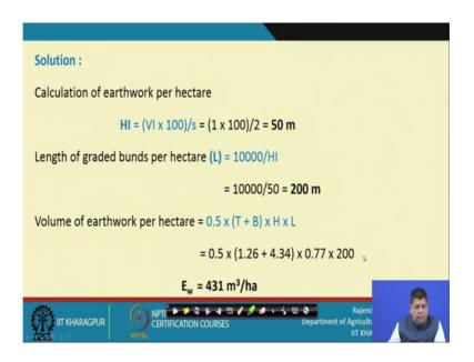
So, now we have to in of the second part of this is we have to calculate the earthwork. And for earthwork per hectare we required horizontal interval and we already know the relationship between horizontal interval, vertical interval the value of vertical interval is given. So, horizontal interval comes out to be 50 meters to length of graded bund per hectare is 10000 square meters divided by H I in meters that, is around 200 meters.
