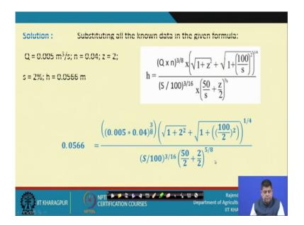
And once we have obtained this. When once we have obtained, we can substitute all the values because Q is known n is known z is known s is known and h is known we can substitute in this. So, only unknown is capital S or channel bed slope. So, by putting all the values in this equation and solving, we get s equal to or the channels slope equal to 0.0674 percent
