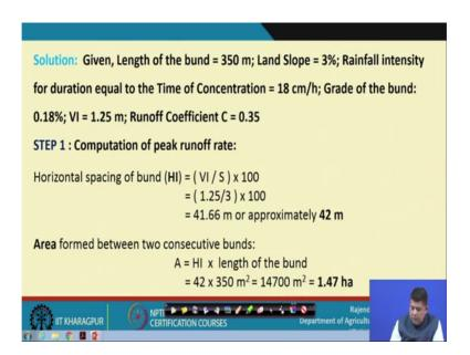
Now, just to have a check on the data which is available with us length of the bund is given as 350 meters, land slope is given as 3 percent, rainfall intensity for duration equal to time of concentration is given as 18 centimetre per hour. The grade of the bund is given as 0.18 percent vertical interval is 1.25 meters and runoff coefficient C is 0.35.
