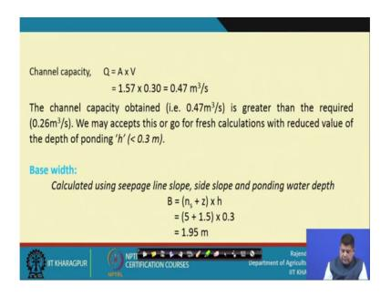
So that means, from knowing the velocity and area we can calculate Q which, is here. The channel capacity obtain 0.437 is greater than the required. We require only this much and we are getting much greater. So, we may accept this or we may go and reduce the value of depth of ponding h. So, that is what I mean if you assume the value you have to do iterate it. So, that iteration process is there, but we are not doing, but because you can do that anywhere and once A h is calculated.
