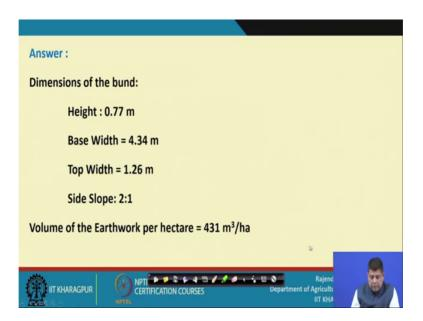
So, the final answers are dimensions of the bund height equals to 0.77 meters, base width 4.34 meters, top width 1.26 meters side slope 2 is to 1 and volume of earthwork per hectare 431 cubic meter. So, this is what the answer will be.
