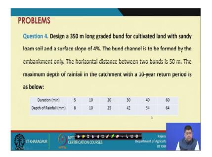
So now we go to the last problem design a 300 metre long graded bund for a cultivated land with sandy soil sandy loam soil surface slope of 4 percent bund channel is to be formed by embankment only. The horizontal distance between 2 bunds is 50 meters the maximum depth of rainfall in the catchment with 10 year return period is given below. So, duration versus depth of rainfall relationship is given here.
