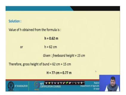
And once h is known then; obviously, we have to get the total gross height of the bund the free board value is given is 15 centimetres. So, the gross height of the bund is calculated height plus 15 centimetre that is 77 centimetre or 0.77 meters. That is the value of h we have obtained.
