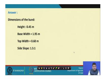
We obtained are the height is 0.45 meters base width is 1.95 meters top, width is 0.6 metres and side slope that is soil dependent, which we started with this 1.5 is to 1. So, this is how we have designed a handled the particular problem.
