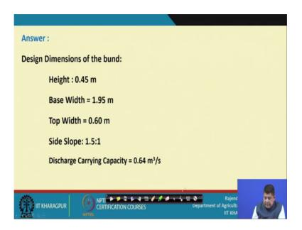
So, thus in this case that final answers are height of bund 0.45 metres base width 195 top width 0.6 side slope 1.5 is to 1 discharge capacity is 0.64 cubic meter per second whichis slightly higher, but we accept that.
