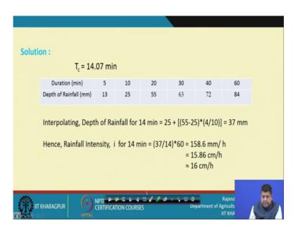
So, if you look at the table the value is given for 10 and 20. We have to obtain for 14 so; obviously, we can we can always interpolate in between these 2. So, interpolating we get 25 plus 55minus 25 by 10 times 4. So, total it comes out to be 37 millimetres.
