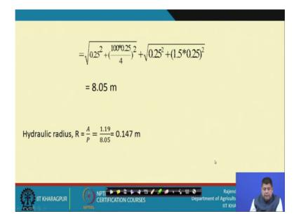
So; obviously, then it is a just A iteration. So, we will go and change the value, calculate A calculate P, then calculate hydraulic radius which new value comes out to be 0. 147.
