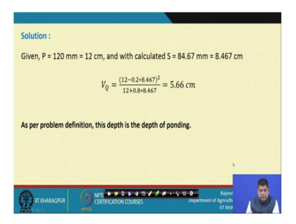
That is precipitation is given as 120 millimetres or 12 centimetre. And value of S we have calculated is 8.467 centimetres. We are converting into centimetre because the value of P and S required for in the curve number method are in centimetre.
