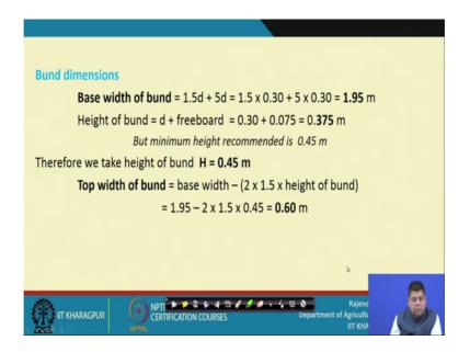
So, the bund dimensions the discharge is handled. So, the bund dimensions can be calculated the base width of bund we know how to calculate height of the bund we know how to calculate, then top width of bund we know how to calculate. So, once H is known everything else can be calculated easily.
