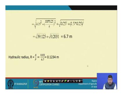
We calculate the hydraulic radius which comes out to be 0.1234 meters and once hydraulic radius is known.
