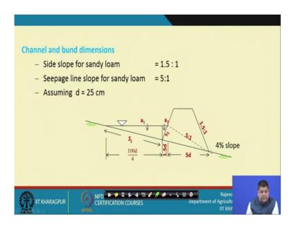
So; that means, we have to handle this discharge. And then rest of the things, side for sandy loam is known 1.5 is to 1 for seepage line. For sandy loam is 5 is to 1. We assume a depth of 25 centimetres and like previously, we have solved this problem we can go ahead and get the cross section etcetera
