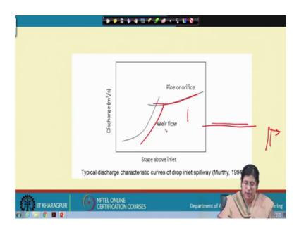
So, now this is you can see a typical discharge characteristic curve of drop inlet spillway so, here the first part is come where flow prevails and the second flow the pipe or orifice flow prevails. So, this is the weir flow and here, an intersection point is located in between two.
