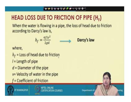
Now, coming to a hydraulic design, so, here we have to consider the friction loss in the pipe and other kind of losses. So, this is in general it is taken from the flow through conduit or the pipe flow. So, as you know the when the water is flowing through the pipe it is in general governed by the Darcy's law.
