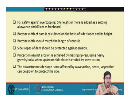
Now, to come back the safety against overtopping 5 percent more height should be added as a settling allowance and which it should kept as 60 centimetre as a free board. And the bottom width of the dam is calculated on the basis of slide side slopes and it is height.
