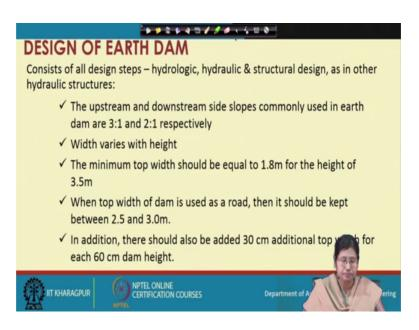
So, now coming to the design of earthen dam, it consists of all design steps that is hydrologic design, hydraulic and structural design and any kind of hydraulic structure. Now, coming to how we can make a design of the earthen dam. So, the upstream and downstream side slope is commonly used in earth dam at a 3 is to 1 or 2 is to 1 slope.
