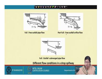
So, here so three different conditions are plotted so, here when S n is when the natural slope is less than the slope of the channel so, the free outflow or the pipe flow prevails. When the opposite is true so, when the slope is greater than the natural slope partly full free outfall orifice flow condition prevails and when this slopes are equal. So, full outfall submerged by flow condition prevails.
