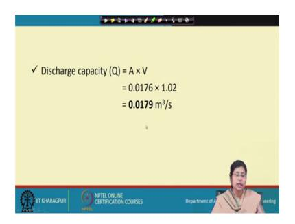
So, here comes the cross sectional area. And now, the discharge capacity is nothing but a function of the cross sectional area and the velocity which is then we multiplied here and getting the discharge capacity of the pipe that is it.
