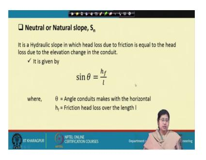
Now, coming to the neutral or the natural slope, it is a hydraulic slope in which head loss due to friction is equal to the head loss due to the elevation change in the conduit. So, it is given by cos sin of the angle that conduits makes with the horizontal. So, here so it is a function of friction head loss over the length l. So, sin theta is the function of h f divided by l.
