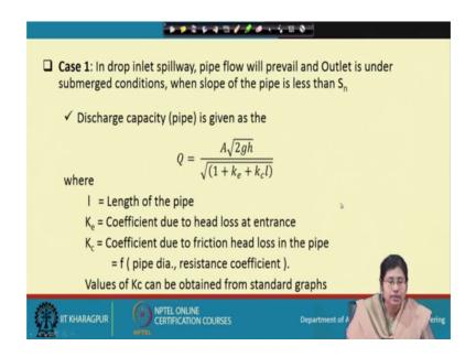
Now, coming to case 1, in drop inlet spillway, pipe flow will prevail and outlet is under submerged condition, when the slope of the pipe is less than S n. So, the discharge
