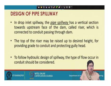
Now, coming to design of the pipe spillway in drop inlet spillway a pipe spillway has a vertical section towards the upstream face of the dam. So, this vertical section is called as a riser and this is connected to conduit passing through dam. The top of the riser maybe raised up to a desired height for providing grade to conduit and protecting gully head. Now to follow hydraulic design of the spillway the type of flow occur in the conduit should also be considered.
