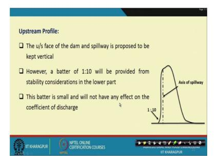
Now, we designed upstream profile, the upstream face of the dam and spillway is proposed to be kept vertical here; however, a batter of 1 is to 10 will be provided from stability point of view in the lower part which is shown here. So, this batter is small will not have any effect on the coefficient of discharge. So, this is the axis of this spillway which is supposed to kept vertical; however, a batter clearance of 1 is to 10 is provided for stability point of view which is shown here.
