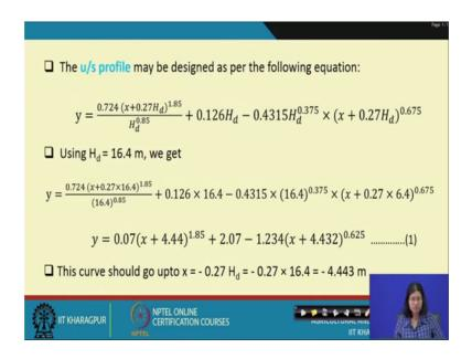
Now, the upstream profile maybe designed using this equation and using H d equal to 16.4 metre we can get a profile shape here and this curve should go up to x equal to minus 0.27 H d which is shown here.
