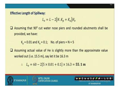
Now, coming to the design of effective length of the spillway where length is given by this formula assuming that 90 degree cut water a nose piers and rounded abutment shall be provided. So, in this case we have from the table the K p value is 0.01 and K a is 0.1. Hence, as the problem given the number of pier was 5. So, n equal to 5 here so, assuming the actual value of H e is slightly more than the approximate value which is worked out here let it say 16.3 metre.
