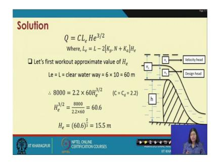
So, first we will study the discharge capacity of the spillway and the length and then one by one we are going to approach this problem. So, first as we mentioned earlier so, H is the height here and H e is the total height which is combination of velocity of approach as well as design head. So, these things we already have in mind. So, the discharge acquired to the constant of the times the L e the length e and H to the power 3 by 2.
