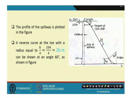
Now, this profile of the spillway is plotted in the figure and a reverse curve at the toe as a is mentioned here h by 4. So, 26 metre can be drawn at an angle of 60 degree as shown in the figure.
