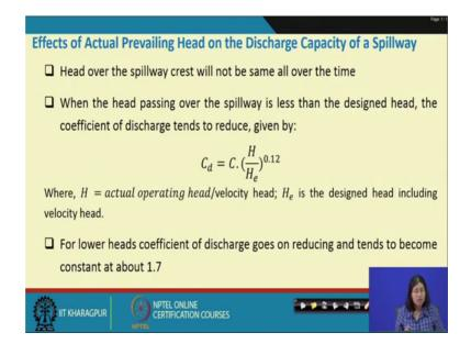
Effect of actual prevailing head on the discharge capacity of spillway. So, head over the spillway crest will not be same at all the time. So, when the head passing over the spillway is less than the neglect design head the coefficient of discharge tends to reduce and in that case it is given by C d equal to C the ratio between H by H e whole to the power 0.12. Where H is actual operating head or the velocity head and H e is the design head including the velocity head.
