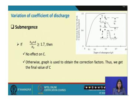
Now, coming to the submergence problem, if this is a case is showing where the submergence problem can arise. So, here h d where d is the depth of submergence and h d plus d again h d is the design head here and d is the depth of this profile and divided by H e is the total again the sum of H a and H d is greater than 1.7. Then what happens? There is no effect on C or the coefficient of discharge, otherwise a graph is used to obtain a correction factor thus we can get a final value of C.
