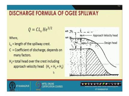
Now, the discharge formula so, this is the sample spillway where H as I explained earlier is the height between the ground and height of the upper profile of the spillway. H d is the design head, H a is the velocity of approach or it can be explained as approach velocity head and H e is the summation of H a and H d, that is sum of velocity of approach as well as the design head. Here it is the total the tail water and is the water level of the upstream surface of the spillway.
