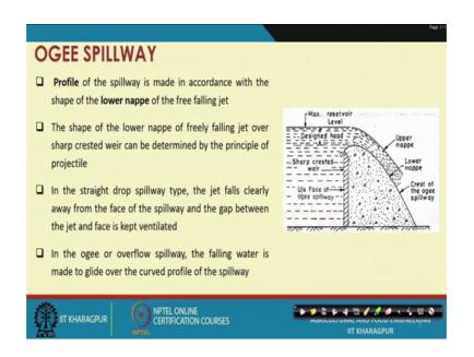
Now, coming to the next slide, now the profile of Ogee spillway is made in accordance with the shape of the lower nappe of free falling jet. So, this is the kind of structure in the Ogee spillway and here this is the upper nappe, the surface of the water profile and the lower nappe, which touches the spillway structure and this one is the crest of the spillway. The shape of the lower nappe of freely falling jet over the sharp crested weir can be determined by the principle of projectile.
