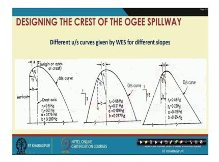
Now, as I was mentioning the different upstream shaped curve are given by WES for different slope. So, this is the example of vertical face where it is kept at a 90 degree angle and here r 1 the radius is 0.5 of H d, r 2 is 0.2 of H d, a is the this gap which is given by point 1.75 of H d and b the breadth is 0.282 of H d. So, these are the kind of dimension is given for the vertical face of the Ogee spillway.
