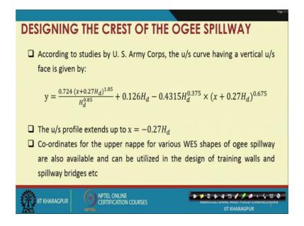
Now, coming to the next design step so, now, we will going to learn the vertical and horizontal coordinates and how to design the shape crest profile of the spillway. So, y is function of x, where it is and again an empirical formulation. So, y is 0.724 multiplied by x plus 0.27 H d, where H d is the design height over the spillway crest whole to the power 1.85 divided by H d. So, this is the kind of equation we are going to use for designing of y given we have x values.
