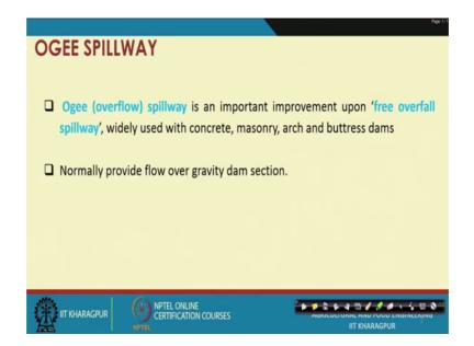
So, what is Ogee spillway? Ogee spillway is an important improvement upon free overfall spillway that is the free fall and widely used in concrete, masonry, arch and buttress dams. Normally, it provide flow over gravity dam section.
