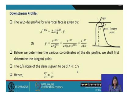
Now, coming to the downstream profile, the downstream profile is given by following formula. So, before we determine various coordinates of downstream profile we first determine the tangent point. The downstream slope of the curve is given as 0.7 horizontal and 1 vertical so, dy by dx is 1 upon 0.7.
