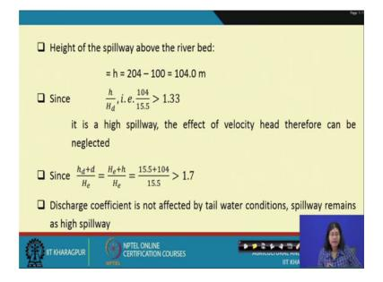
Height of the spillway above the river bed. So, here h is 204 which is this figure here. The height of the spillway crest is kept RL as 204 metre and average river bed level at the site is 100 metre. So, the total height of the spillway crest is h 204 subtracted by 100 is total now 104 metre.
